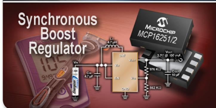
The diagram shows an MCP16251/2 Synchronous Boost Regulator circuit with a 3.3V output and 100 mA current. Components include a 4.7 μF capacitor, a 4.7 μH inductor, and resistors of 976 kΩ and 562 kΩ.
